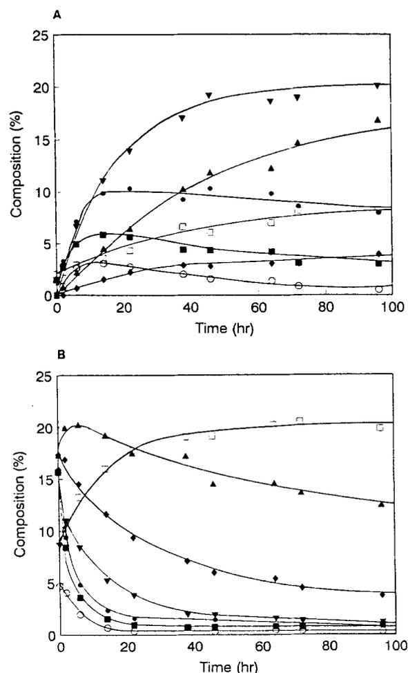
Figure 6. Time course assay of BOS production. Panel A shows change in the concentration of glucose (□), maltose (▲), maltotriose (◆), maltotetraose (▼), maltopentaose (●), maltohexaose (■), and maltoheptaose (○) in the liquefied starch solution as BOS is synthesized by the action of BLMA. Panel B shows increase of isomaltose (□), isopanose (◆), panose (▲), BDP4 (▼), BDP5 (●), BDP6 (■), and BDP7 (○) as the reaction proceeded.
