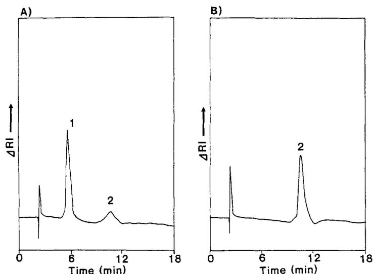
Figure 4. High performance liquid chromatography of branched DP4 in the BOS mixture.
