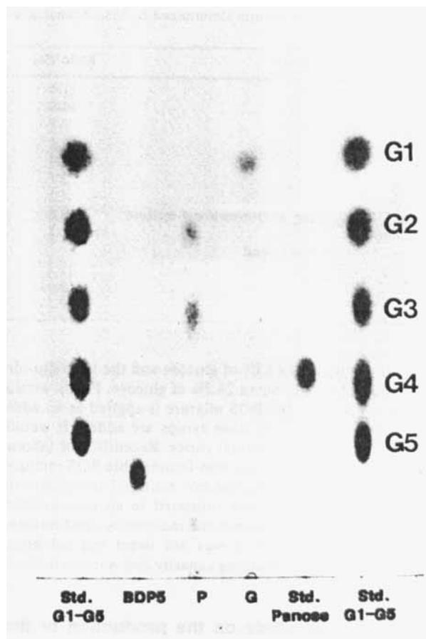
Figure 5. Thin layer chromatography of branched DP5 in the BOS mixture.
