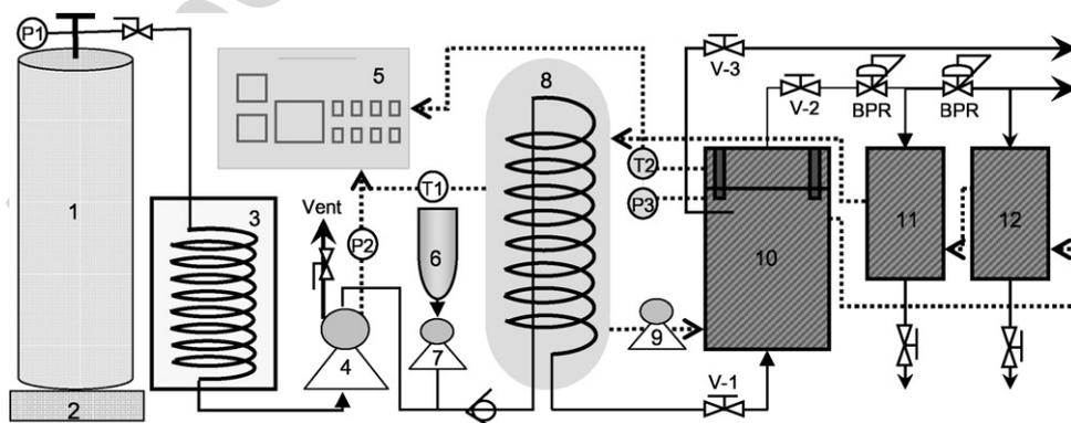
Fig. 1. Schematic diagram of the supercritical CO<sub>2</sub> extraction system: 1, CO<sub>2</sub> cylinder; 2, electronic balance; 3, chiller; 4, CO<sub>2</sub> pump; 5, controller; 6, cosolvent reservoir; 7, cosolvent pump; 8, heating bath; 9, circulation pump; 10, extractor; 11, separator 1; 12, separator 2; V1, valve 1, V2, valve 2; BPR, back pressure regulator; dotted lines, water line; solid lines, CO<sub>2</sub> line.
